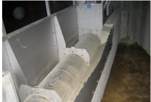
ROTAMAT® Storm Screen RoK 2 with an integrated gauging weir for overflow measurement
